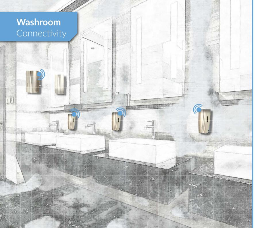
Technology enables direct communication from individual dispensers to assess usage, fill level and battery life. This allows your teams to be alerted when dispensers are close to running out of consumables.
