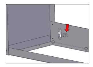
**Vertical** adjustment is carried out by slightly loosening the anchor bolts and sliding the cabinet up or down.
